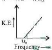
where work function depends on the type of material. If the frequency of incident radiation is greater than  $\upsilon_0$  only then the ejection of photoelectrons start. After that as frequency increases kinetic energy also increases
